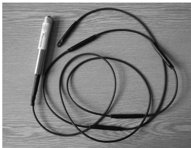
Figure 1. M-Log5W data logger ( www.GeoPrecision.com ) and attached thermistor string.
