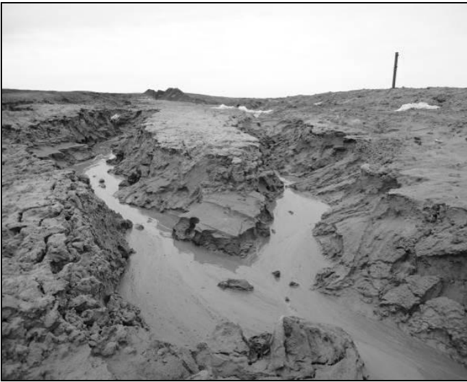
Figure 1. The erosion of sandy silt grounds of the seasonally thawed layer upon removal of the peat layer
