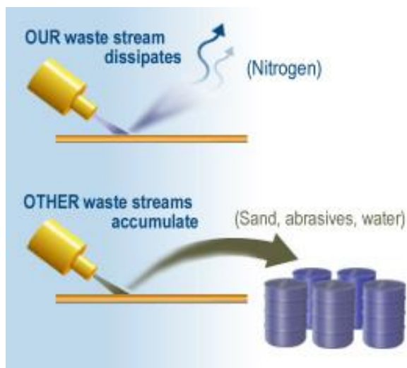
Figure 2. Removal of coatings by a supersonic jet of a cryogenic agent. A liquid nitrogen jet is ejected at high pressure, cuts solid material like a hot knife cuts butter and then vanishes in the air.
