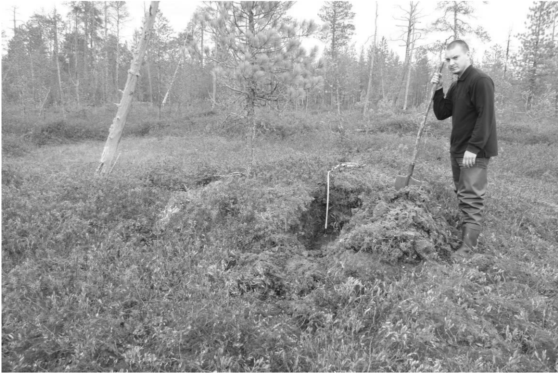
Figure 2. Determining the thickness of thawed and frozen layers.
