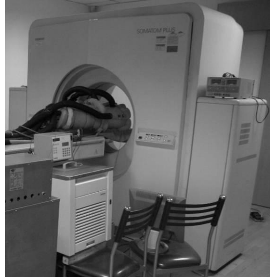
Figure 2. The CT Scanning System with triaxial test apparatus
