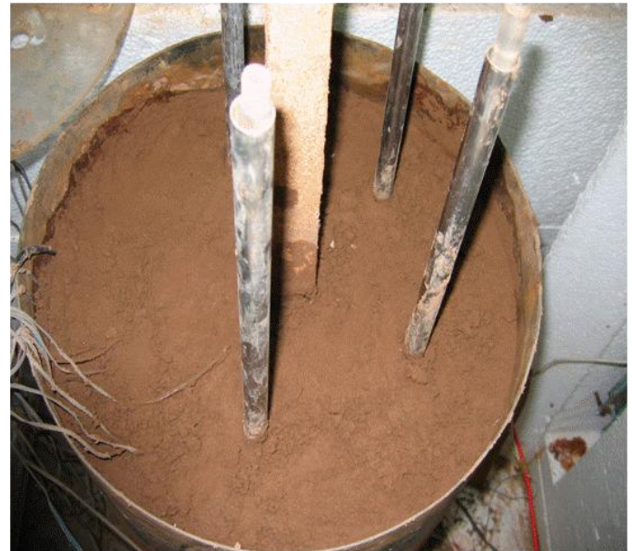
Figure 1. Model pile test assembly picture
