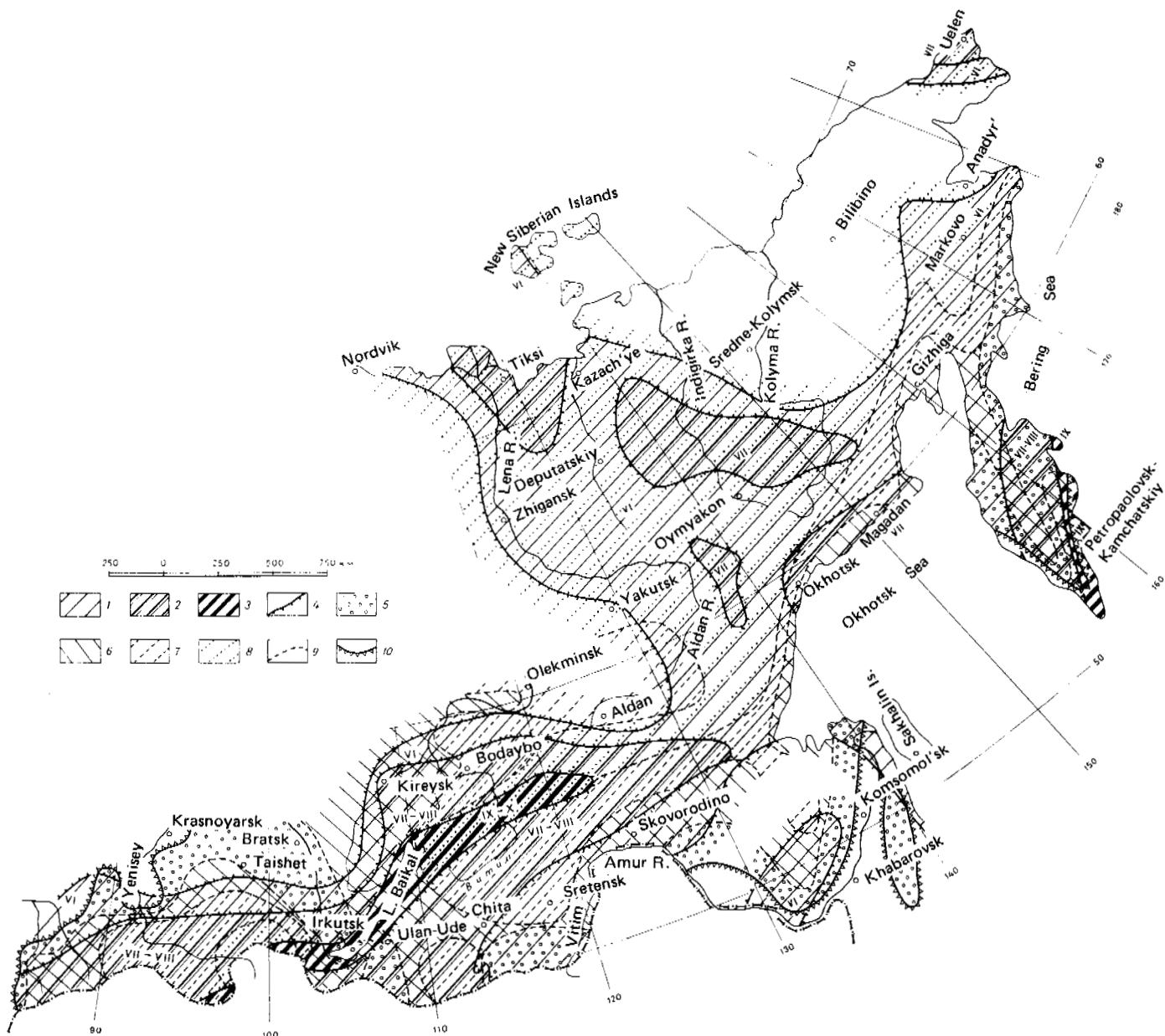
FIGURE 2 Diagram showing seismic zoning of USSR permafrost area. Seismic regions (1-4): 1--intensity of VI; 2--intensities of VII and VII + VIII; 3--intensity of IX and higher; 4--limits of seismic regions (marks on side--in direction of regions of decreased intensity). Permafrost regions (5-10): 5--individual islands of plastically frozen and pseudo-thawed soils; 6--insular type of permafrost with plastically frozen and pseudo-thawed soils; 7--permafrost with islands of taliks, with complexes of solidly frozen and plastically frozen soils; 8--continuous permafrost with solidly frozen soils; 9--limits of permafrost regions (name of regions and condition of soils--according to prevalence); and 10--limits of permafrost area.
