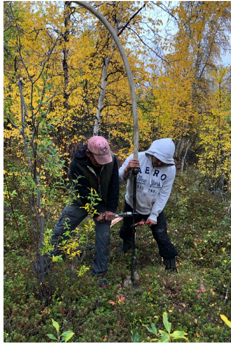
Water jet drilling at Reindeer Station, NT, by monitors from the Inuvik Community Corporation (September 2021). Photo: Alice Wilson (NTGS).
