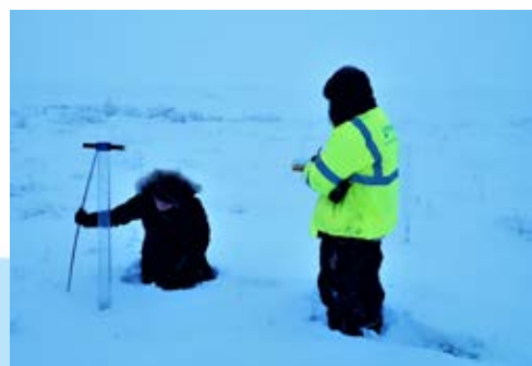
Left: Alice Wilson and Mary Cockney (ILA, Environmental Monitor) collecting snow depths and densities. Right: Snow cat at a compaction site near the ITH (both January 2021).
