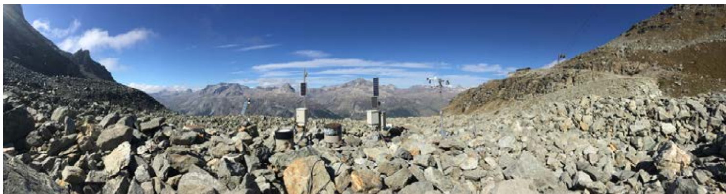
Deep boreholes (60 m), measurement stations and MeteoStation on top of the rock glacier Murtèl in the Swiss alps at 2670 m asl. TSP measurements ensured some GTN-P data entries in 2020. Photo: Jeannette Nötzli.
