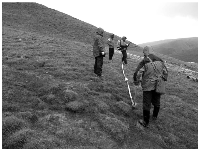
GPR sounding of permafrost near Wenquan. (Photograph provided by Guan Gyue Liu)
