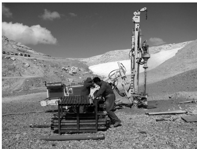
View of the drilling operation for the 100 m deep borehole at Sommeiller (3000 m a.s.l.) in Upper Val Susa (Western Alps, Piemonte) where a new permafrost monitoring station has been installed in the framework of Permanet. (Photograph provided by Luca Paro)
