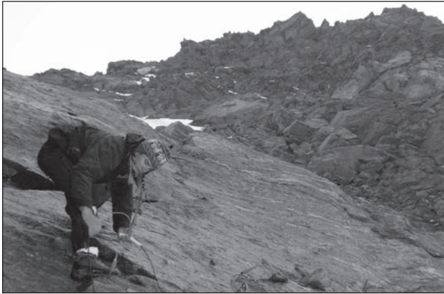
Installation of an ERT-transect for permafrost monitoring in a creeping north-exposed rock wall at 3100 m a.s.l., Steintälli, Valley of Zermatt, Switzerland. (Photograph provided by Michael Krautblatter)
