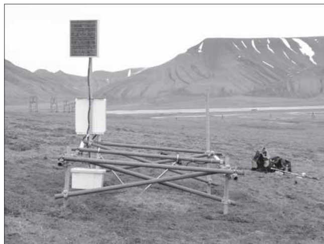
Field station monitoring active-layer gelifluction processes, Endalen, Svalbard, installed in August 2005. Photograph by Charles Harris.
