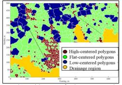
Data-driven delineation of polygon types at the NGEE-Arctic Barrow, AK study site. Multiple data types and a statistical approach were used to document the existence and importance of functional zones, or groups of polygons that have unique distributions of above and below ground properties that influence carbon fluxes.
