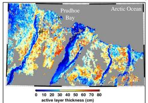
1992-2000 average Remotely Sensed Active 1992-2000 average Remotely Sensed Active Layer Thickness (ReSALT) for the Prudhoe Bay area on the North Slope of Alaska derived from the European Remote-Sensing Satellite (Liu et al., 2012).
