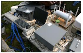
Measuring  $\delta$ 13C of ecosystem respiration using the Picarro G2121- i
