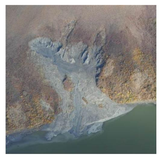
Figure 1: Aerial photograph of a retrogressive thaw slump on the Noatak River in the Noatak National Preserve, September, 2012. The escarpment of this slump retreated as much as 30 m between July 2011 and September 2012, releasing approximately 50,000 m3 of material as the slump grew to cover 3.5 ha
