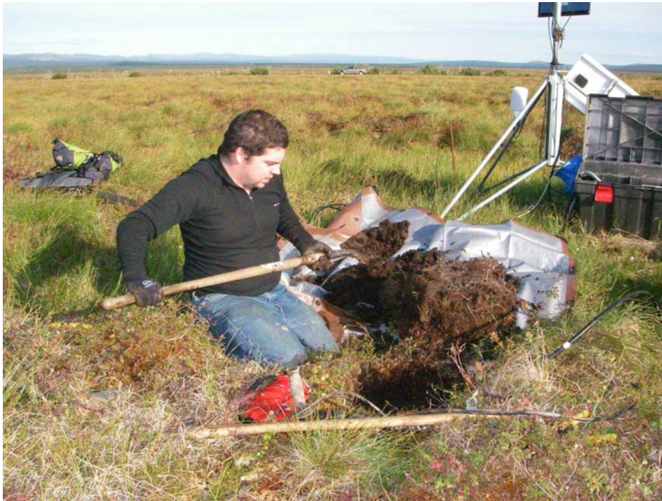
Research Engineer Bob Busey excavates a new shallow borehole to replace soil thermistors near the Council CALM grid, Seward Peninsula (photograph provided by J. Cherry).
